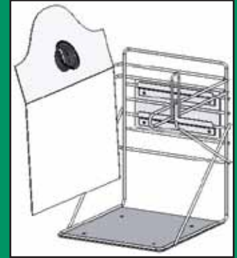
Spool holding bags mounts to one side of rack. Bag opens to prong on other side to hold open.
